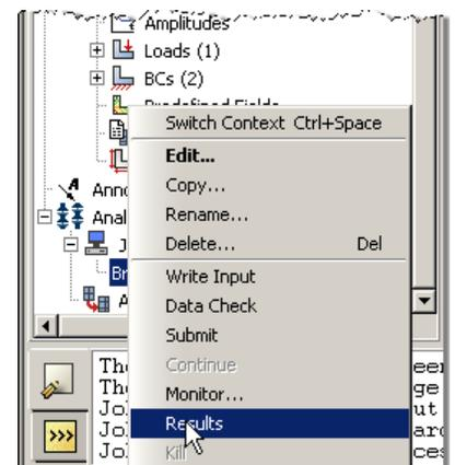
22. To change the output being displayed, in the menu bar click on Results → Field Output
