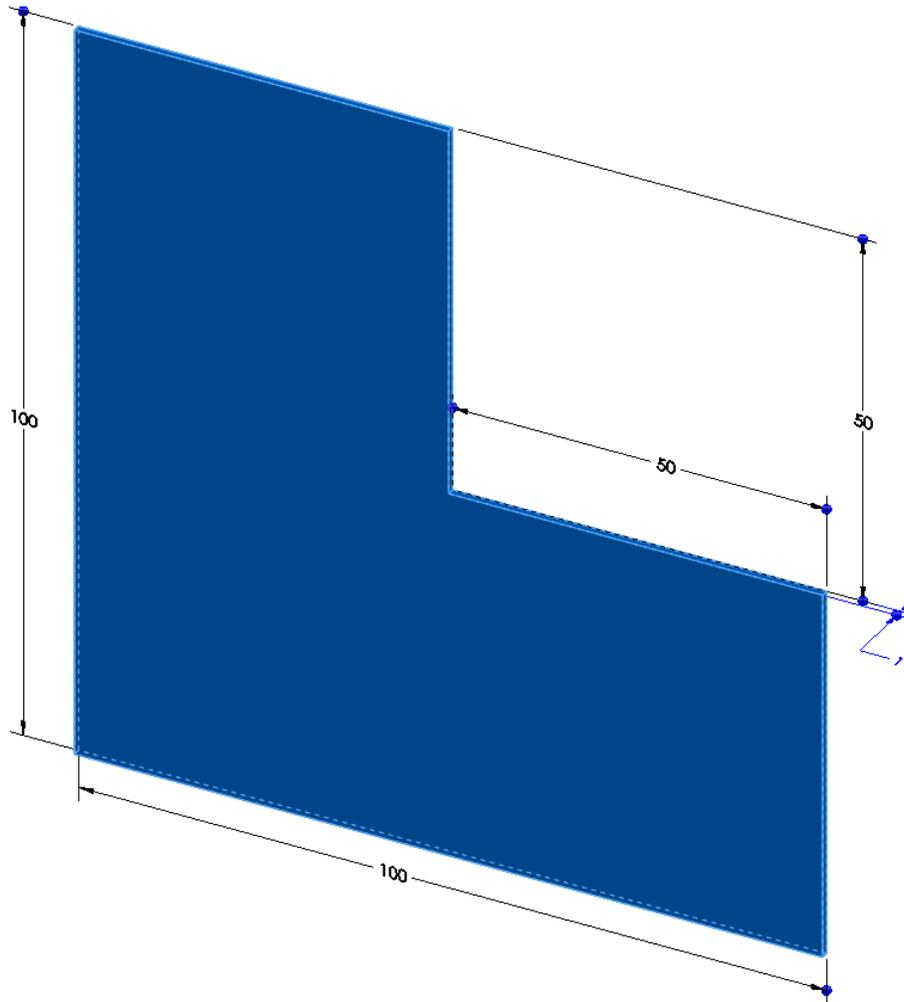
The thin “L-shaped” part shown above is exposed to a temperature of  $20\text{ }^{\circ}\text{C}$  on the two surfaces of the inner corner, and  $120\text{ }^{\circ}\text{C}$  on the two surfaces of the outer corner. A heat flux of  $10\text{ W/m}^2$  is applied to the top surface. Treat the remaining surfaces as insulated.
