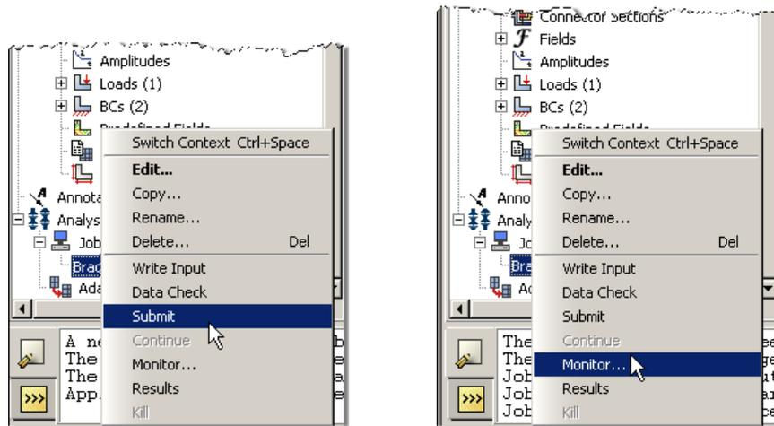
In the Monitor window check that there are no errors or warnings. If there are errors, investigate the cause(s) before re-solving
